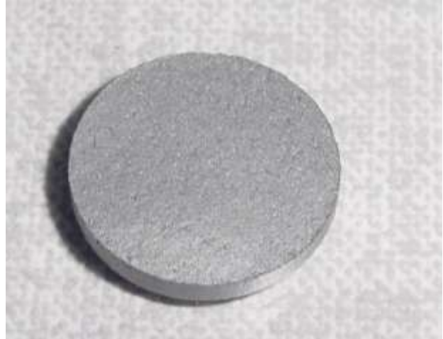
Fig. 3.7: Photograph of pressed-powder UC x target
