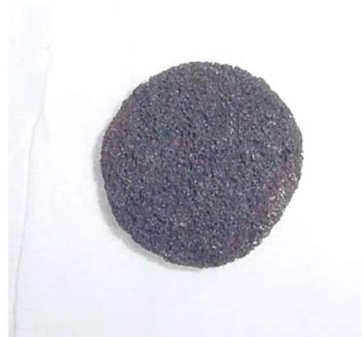
Fig. 3.8: Photograph of UC 2 coated RVC fiber target
