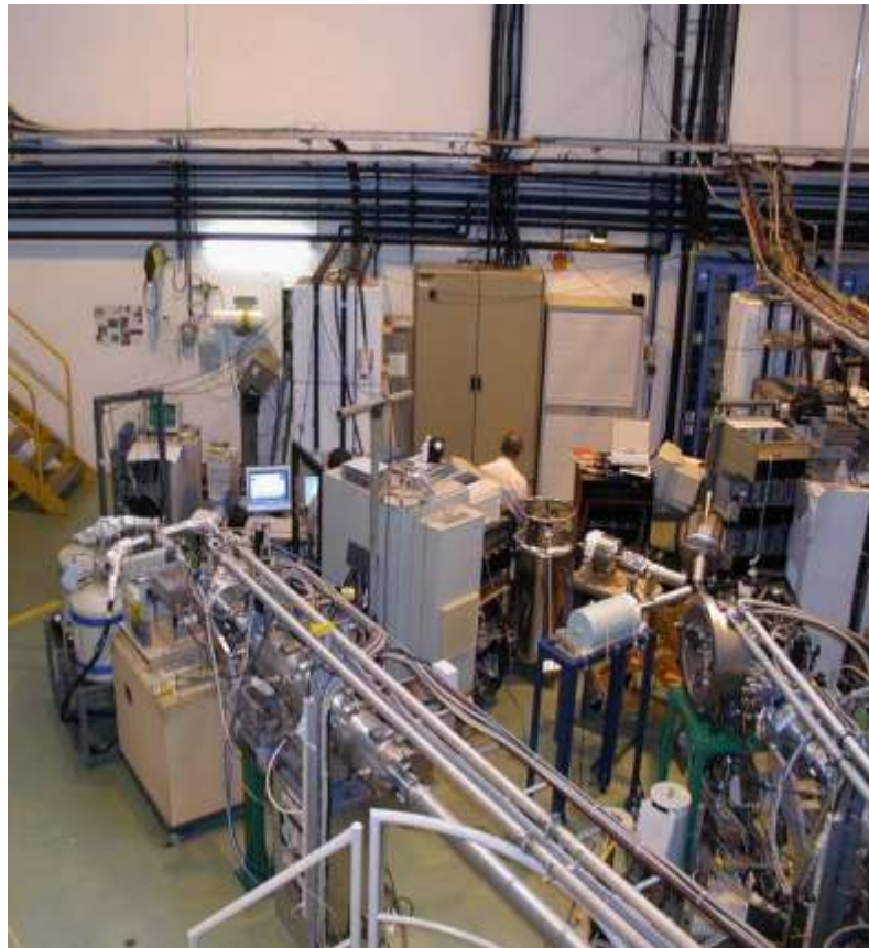
Fig. 3.17: Beam line LA1 (left) with tape station and \gamma -detectors
