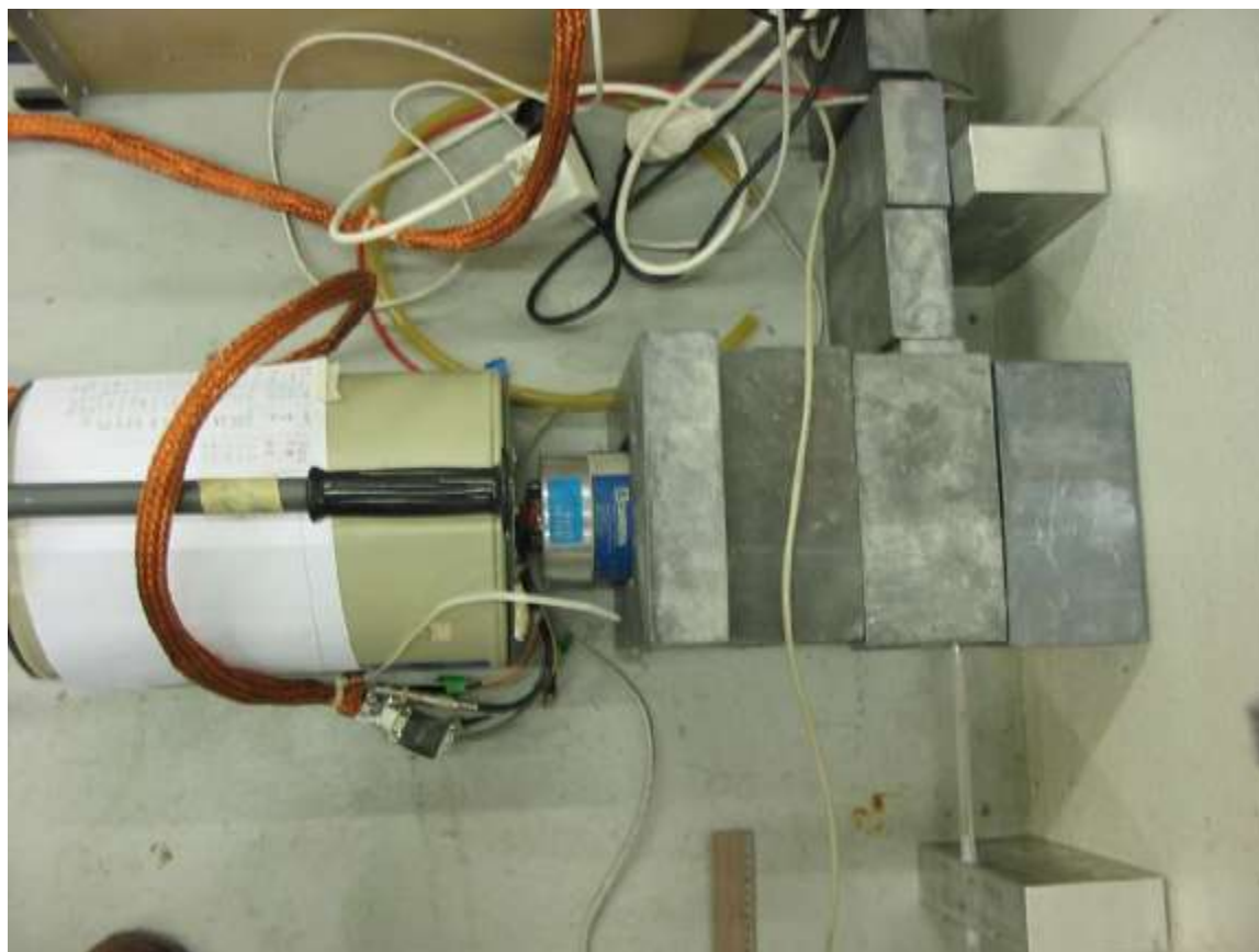
Fig. 3.4: \gamma -setup with 2cm collimator (not visible) and quartz tube
