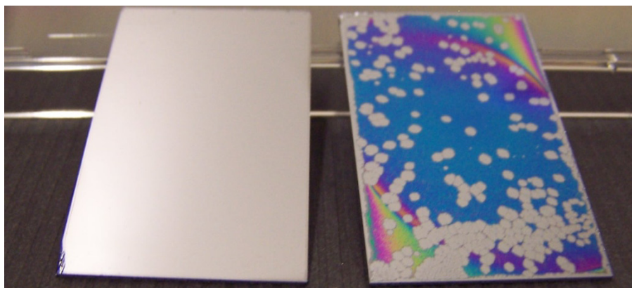
Figure 1.1. Delamination of polystyrene on silicon wafers. Polystyrene ( M_w = 25 kg/mol) was spin-coated onto Si wafers (1 wt% in THF, 4000 rpm, 15 s). The left wafer was just coated, whereas the right wafer was annealed at 130 °C for 1 h.
