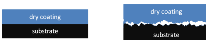
Figure 1.4. Scheme of coating application onto a substrate. Left: atomically flat interfaces; right: rough interfaces, not filled by the coating.
