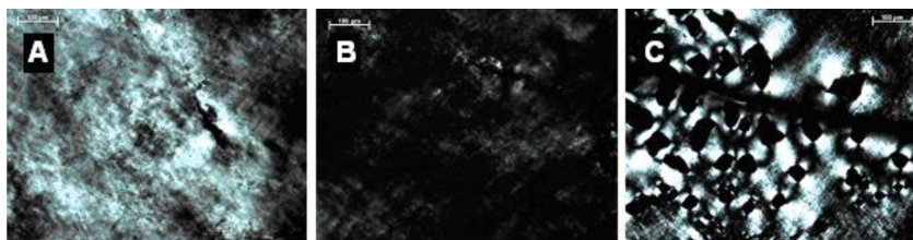
Figure 6.20.: Polarization optical microscope images of OPBA-4-PEG45 at 105^\circ\text{C} . (A) and (B) show the same position of the sample rotated by 45^\circ . (C) Birefringent nonspecific texture.
