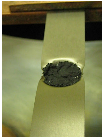
Figure 4.15: Picture of the MgOTa mixture in a dimple boat before evacuating the evaporation chamber.
