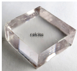
Figure 4.1: Clean calcite crystal with typical rhombohedral shape and birefringence.
