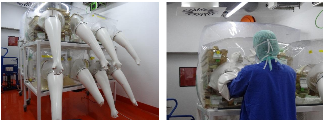
Figure 3. Germ-free mice technology established in the host laboratory. Mice are kept in sterile plastic isolators and handled with gloves attached to isolators.
