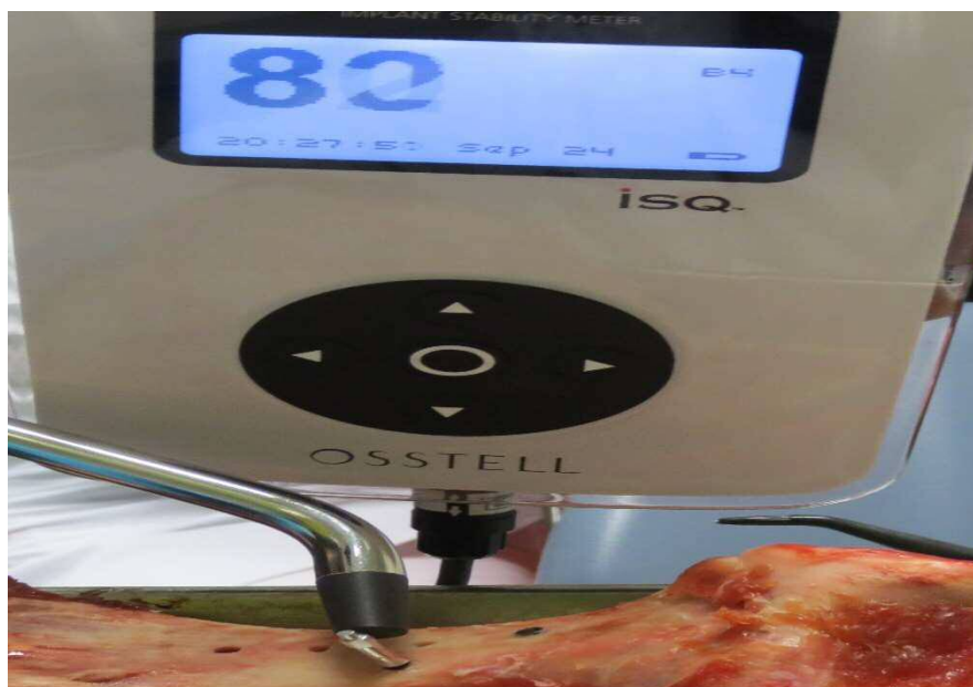
Figure 15: Primary stability measurement by ISQ
