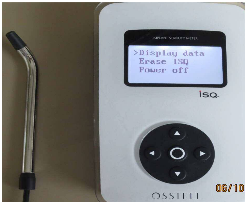
Figure 17: Osstell-ISQ apparatus is using to determine RFA.
