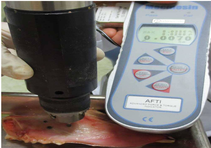
Figure 16: Torque in measurement by handheld torque measuring screw driver (Halmtec, Mecmesin, Germany)
