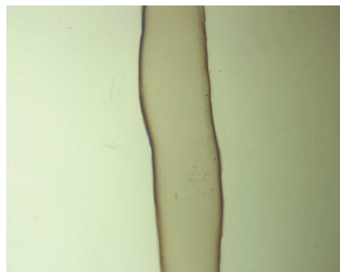
Fig. 4.44.: A 20-bilayer PEM line was plotted directly on the surface of a Si substrate that was freshly cleaned by the Piranha solution (see experimental section 7.9). The picture was taken with a light microscope under bright field.
