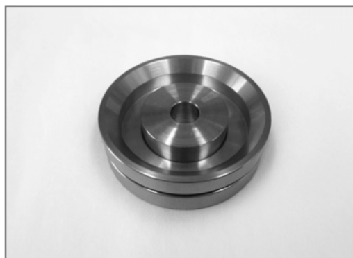
Figure 2.10 Attofluor cell chamber with additional stainless steel ring.
