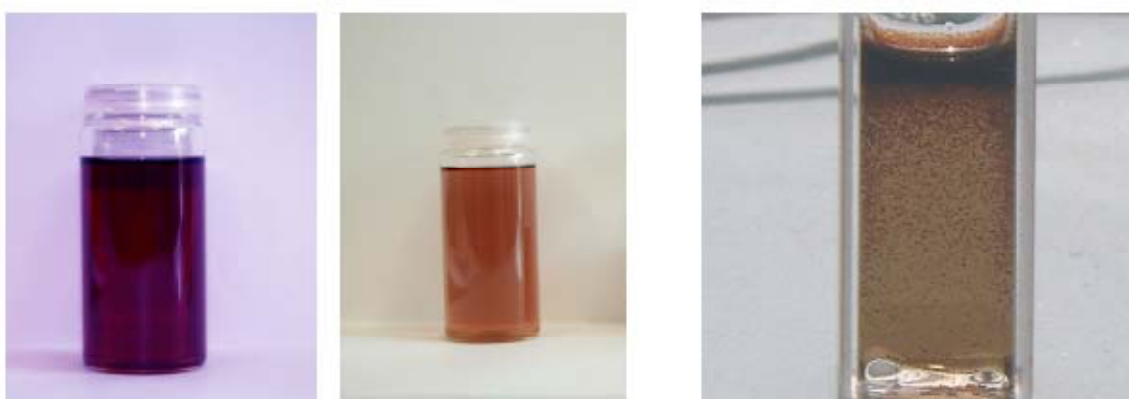
SI 8: Polymer ( 2 ) solutions in dichloromethane (DCM) with Grubbs' catalyst left: directly after mixing. Middle: after 2 h. Right: DCM solution of catalyst after reaction with scavenger resin for 2 h.
