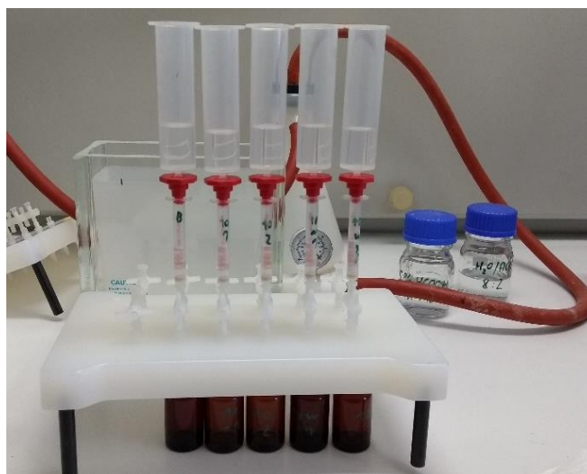
Figure 2.1 The picture shows the cartridges placed onto the upper part of the vacuum manifold during the loading process. The filled sample reservoirs are connected to the SPE cartridges via an adapter. The flow-through is collected in glass vials.
