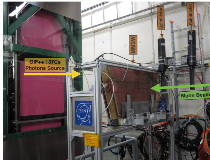
Figure 6.23: The set up for the test at GIF++.
