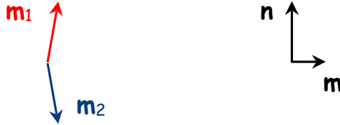
Figure 3.9: Schematic representation of the antiferromagnetic vectors: sublattice vectors \mathbf{m}_1 and \mathbf{m}_2 , and Néel vector \mathbf{n} and total magnetization \mathbf{m} (not to scale).
