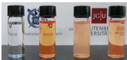
Figure 6. Picture of the solubility change of the hybrids: 1) pure polymer in toluene, 2) hybrid in toluene, 3) hybrid in hexanes, 4) QDs in hexane (from left to right, respectively).
