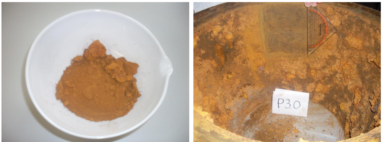
Figure (8-19) Sediment settling amount taken from iron pipe
