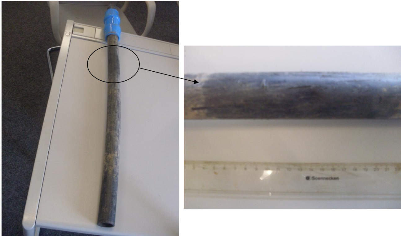
Figure (8-16) Failure case (H-4) for PE pipe crack failure
