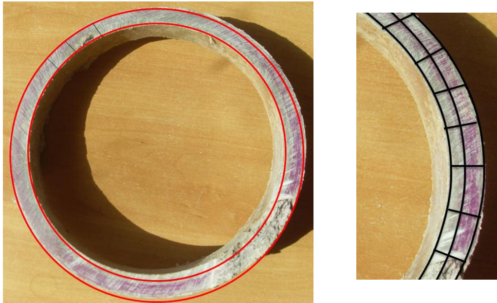
Figure (7-17) The area of maximum cement mortar leaching on each ring section is selected for sub-sampling and further testing.
