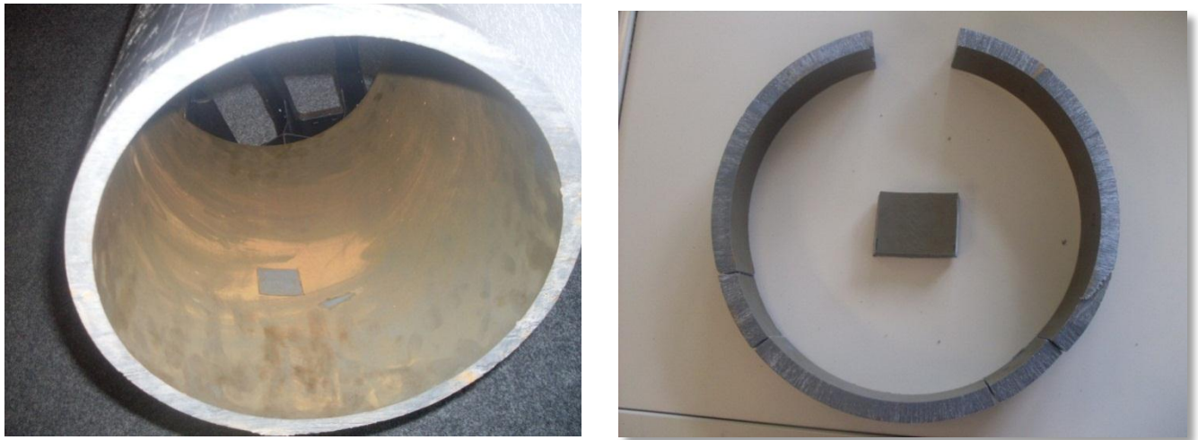
Figure (8-21) UPVC pipe sample preparation
