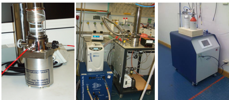
(a) Custom built parahydrogen generator for batch mode generation. Image of the cryostat expander (left) and complete setup (right). The helium compressor (bottom left) and storage bottles for parahydrogen (on top).
