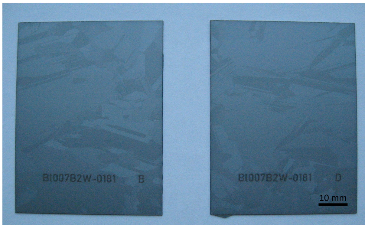
Fig. 4.7 Horizontal neighboring wafers cut from one 156x156 mm 2 sized wafer.
