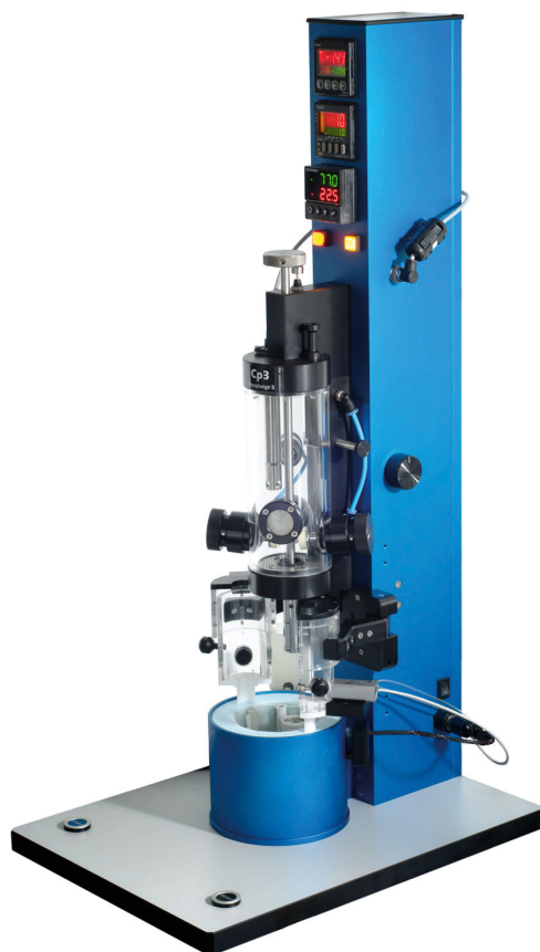
Fig. 2.12 Gatan plunge-freezer CP3. The CP3 as it was used in our laboratory. The displays show ethane temperature, relative humidity and current blotting time. The entire procedure is under controlled atmospheric conditions (image courtesy of Christoph Kuehne).
