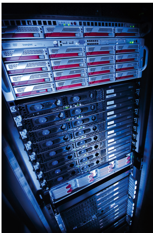
Fig. 2.6 Beowulf cluster at the JGU Mainz. A 358 core AMD Opteron computer cluster located at the Institute of Zoology at the JGU Mainz Germany (image courtesy of Christoph Kuehne).
