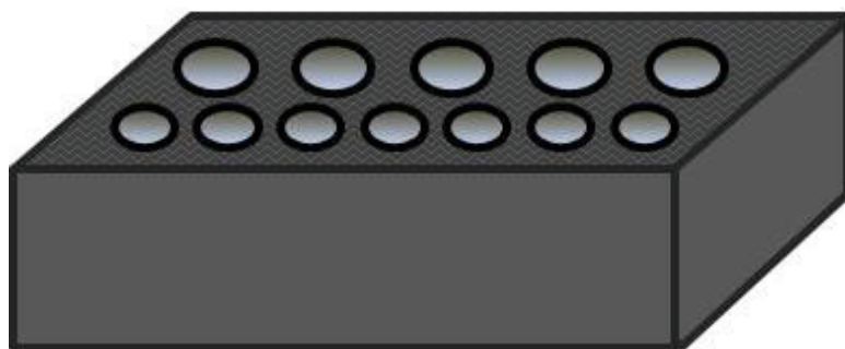
Fig. 2.10 Block staining. The smaller holes take the sample solution and the bigger ones take the staining reagent. At first the grid is placed on the sample and in a second step the grid is placed on the stain. The individual times have to be tested for sample concentration and stain result.
