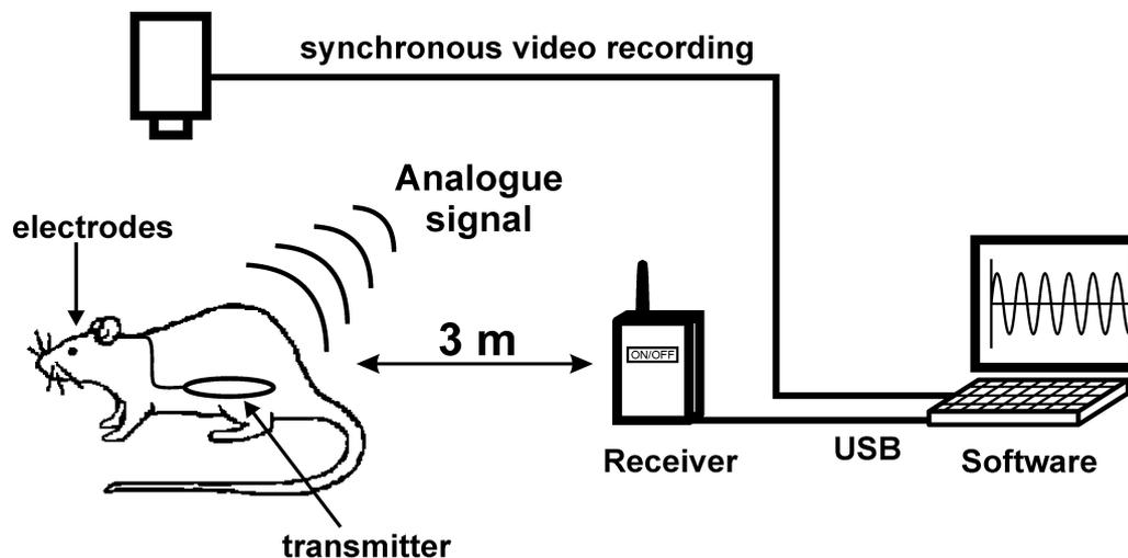
**Figure 11: Overview of the telemetric recording system's main components** (modified from Lapray *et al.*, 2008). The system is composed of the implantable transmitter, a receiver connected to a computer which displays and records the signal synchronously with the video of the freely moving animal.
