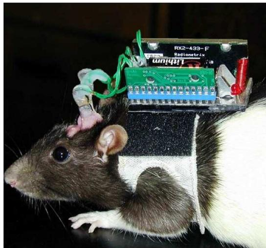
**Figure 9: The backpack style unit.** In this method the animal carries the transmitter directly on its back with the disadvantage of reduced free movements (from Xu *et al.*, 2004).
