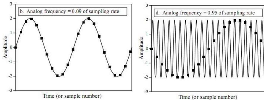
**Figure 10: Nyquist-Shannon sampling theorem.** The left panel shows a proper sampling in contrast to the right panel with the creation of an alias, e.g. a wrong representation of the original analog signal (from Smith, 1997).
