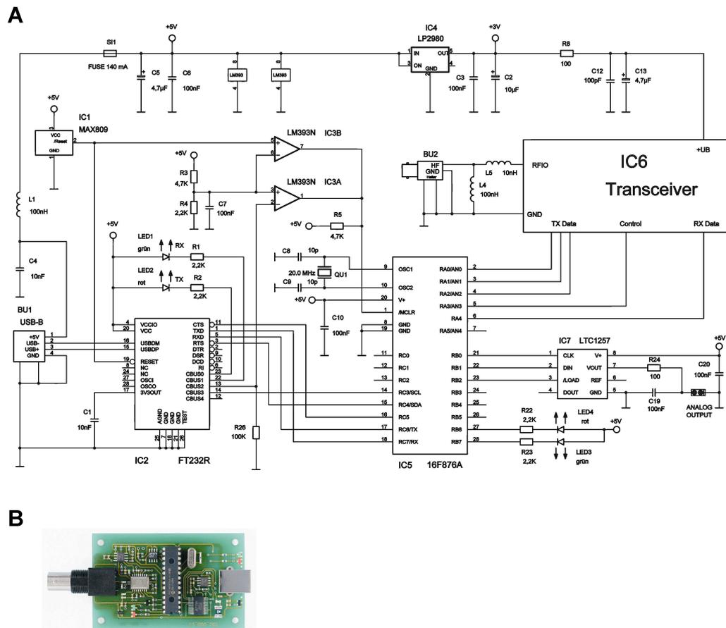
**Figure 13: The receiver.** (A) Electronic circuit diagram of the control interface and (B) photograph of the USB unit (from Lapray *et al.*, 2008).
