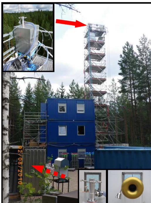
Abbildung 4.2.: Setup of the HORUS instrument on the HUMPPA tower. Simultaneous side-by-side measurements of hydroxyl radicals were conducted at the start of the campaign with two instruments using chemical ionization mass spectrometry (CIMS) and laser induced fluorescence within the forest. The two instrument inlets (shown on the pictures in the lower right corner) were co-located at the side of the container, about 1m a.g.l. .
