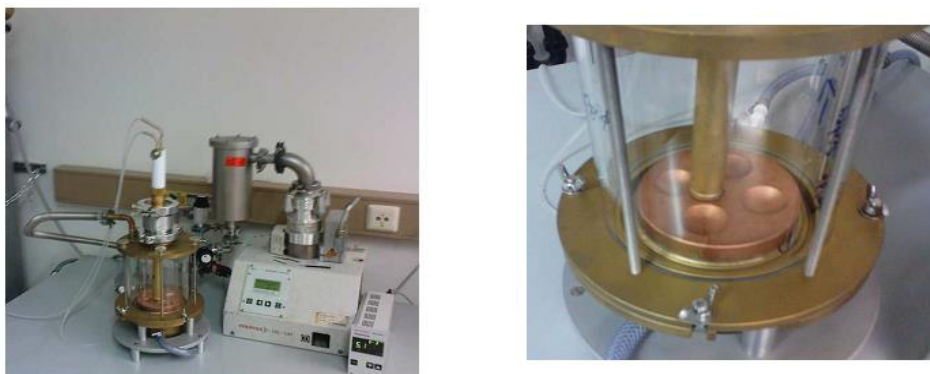
Figure 21 Picture of the arc melting setup taken at the University Mainz.
