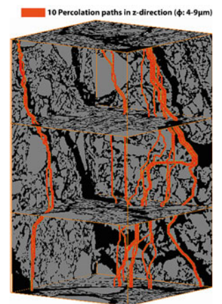
Fig. 6 3D image of main percolation pathway traces (macropores) along z-direction of ROI #1. Soil sample height is 0.74 mm (=1,000 voxels)
