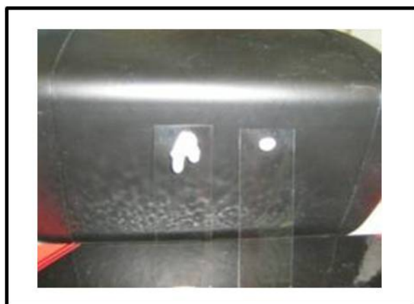
Figure 3.14: Comparison of the paste viscosity, upon addition of either hydrogen titanate- (left) or TiO 2 nanowires (right).
