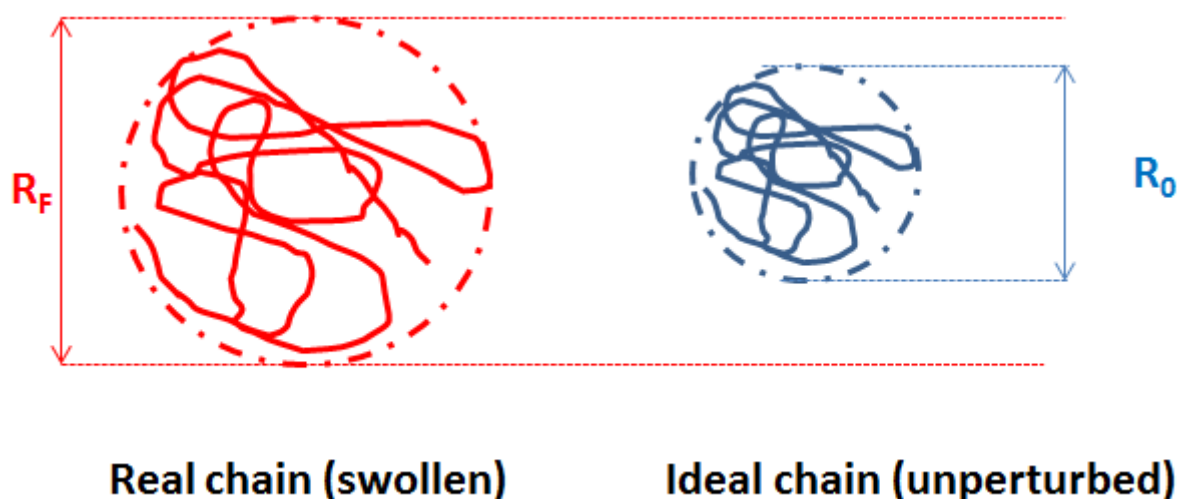
Fig.1.2.1. Qualitative representation of a real chain with excluded volume interactions with a coil dimension, R_F , (left) and an ideal chain with coil dimension, R_0 (right).
