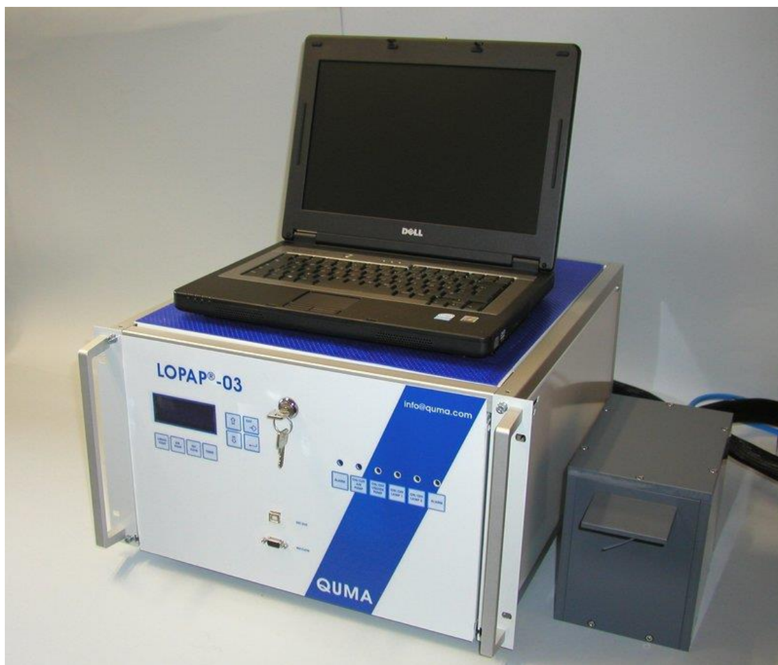
Figure 10. Picture of the LOPAP instrument with external sampling unit (grey box at the right hand side) and a computer for data acquisition is shown. Technical parameters are adjustable at the front panel, like air and liquid flow rate (QUMA, 2006).
