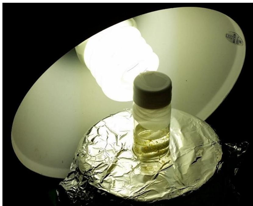
Figure 6.22 A simple photoinitiation set-up using a 23 W household energy saving light bulb.
