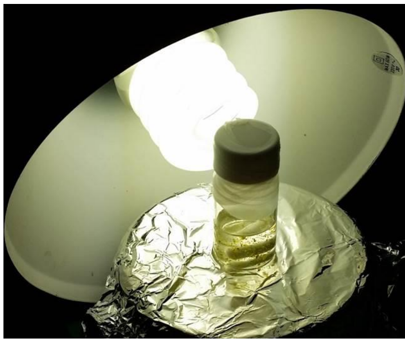
Figure 6.19 Simple set-up of the dehalogenation of haloketones a 23 W household energy saving light bulb.
