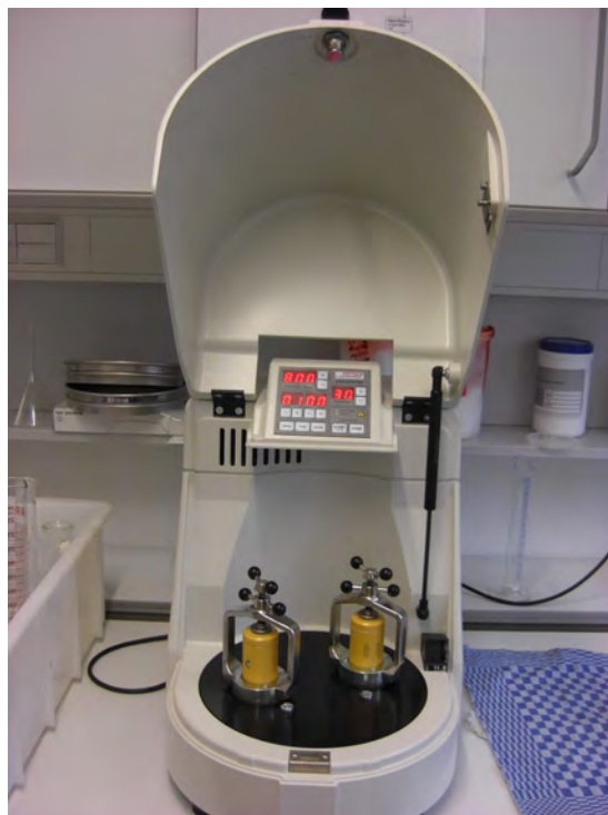
Figure 2.3.2: Fritsch Pulverisette P7 classic line® planetary ball mill
