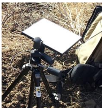
Figure 3.1.6 Image of the ASD Spectralon used during the fieldwork.
