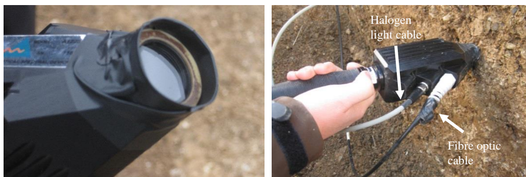
Figure 3.1.4 Image of the contact probe (including a halogen light source together with fibre) and its application in the field.
