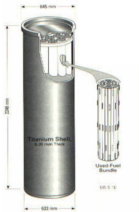
Figure 2: Disposal container design in Canada ( nuclearfaq.ca )
