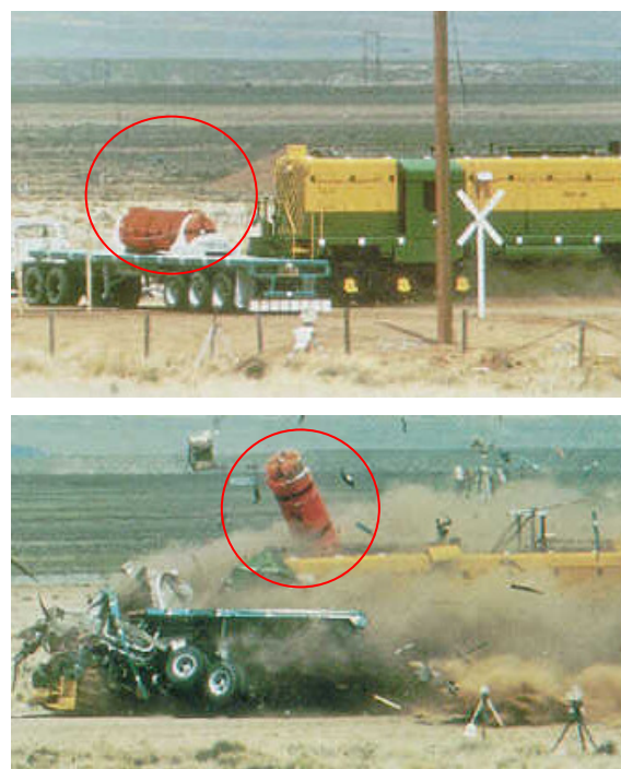
Figure 3: Nuclear waste casks crash tests performed at Sandia National Laboratories in the USA ( nuclearfaq.ca )
