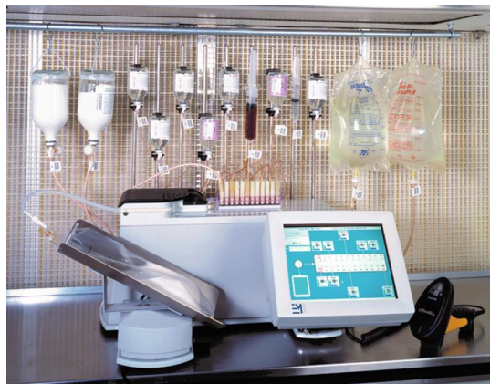
Figure 1: Baxter Exactamix EM2400 Compounder (Figure provided by Baxter International Inc.).
