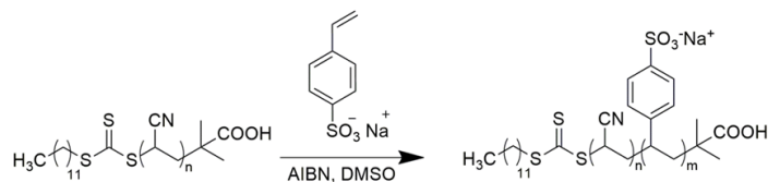
Figure 3: Synthesis route to obtain P(AN-b-SS).
