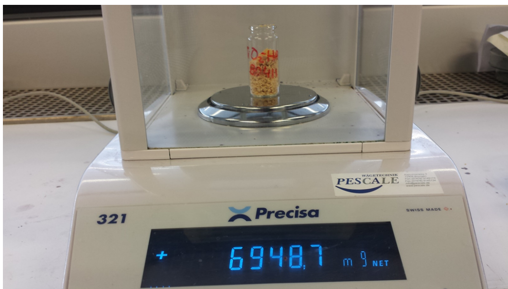
Figure S 5: Photograph of as-synthesized in situ polymer functionalized \text{TiO}_2 particles showing the possibility to synthesize material in gram amounts.
