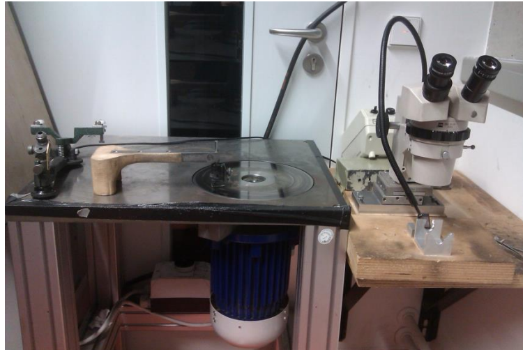
Figure 3.1 Diamond Polishing machine
