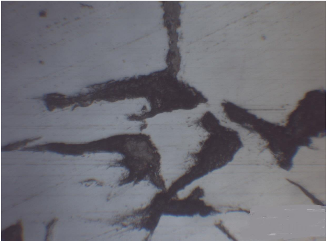
Figure 3.2 Cast Iron disk with cavities which are partially full of silicon carbide abrasive
