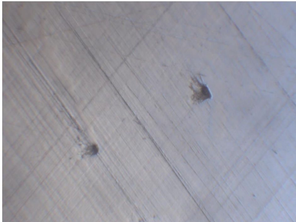
Figure 3.4 Rare diamond inclusions on stainless steel disk after disk re-polishing with 3 micron paste.
