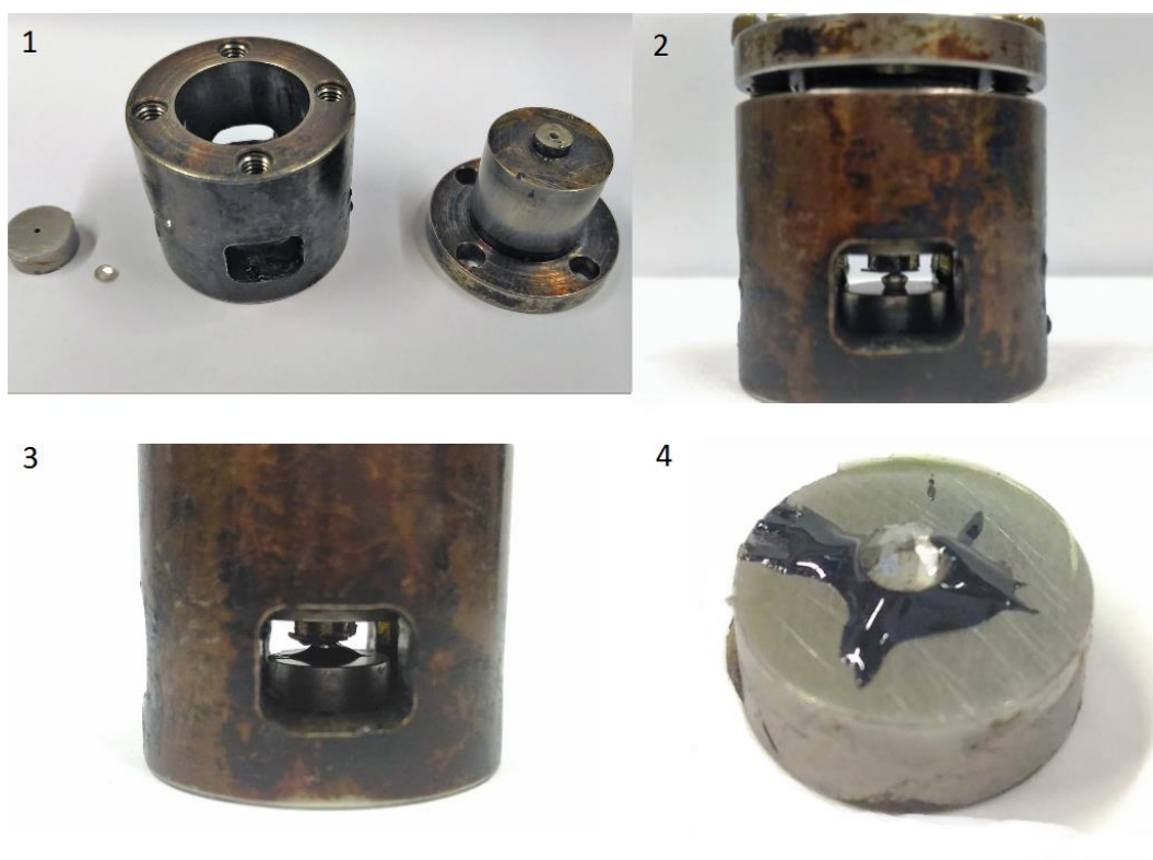
Figure 3.5 A process of diamond gluing into the seat
