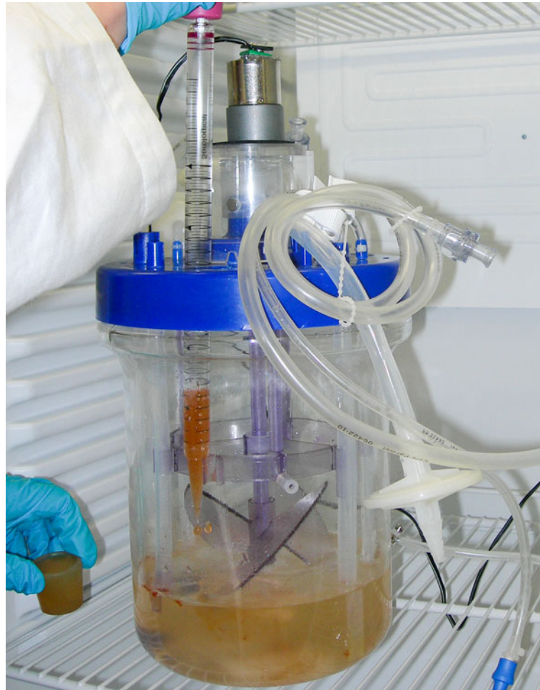
Fig. 20 Commercial bioreactor initially used for primmorph production. Single-use bioreactor from Eppendorf (Wesseling-Berzdorf). The picture shows the addition of a S. domuncula cell suspension to primmorph standard culture medium. This bioreactor allowed to scale up the culture volume to 2 l and to use a whole sponge individual for each primmorph preparation.
