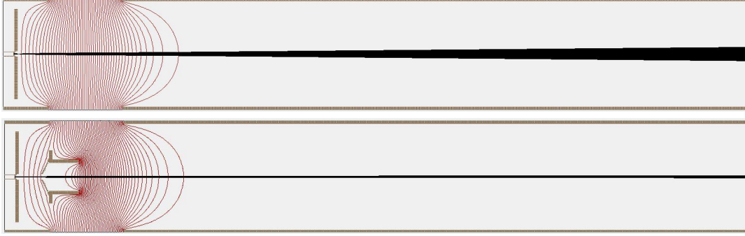
Figure 3.8: Simulations with SIMION [112] of the divergence of the ion beam ( ^{91}\text{Rb}^+ ) over a distance of 1 m behind the surface ion source. The lines of equal potential are shown in red. In the upper figure the ions are accelerated by a high voltage of 28 kV without an additional electrode. The diameter of the beam is about 20 mm after a distance of 1 m. In the lower figure an extraction electrode in Pierce geometry is added 3 cm behind the ion source and biased to 25 kV. In this case a more parallel ion beam is obtained and the diameter after 1 m is less than 4 mm.
