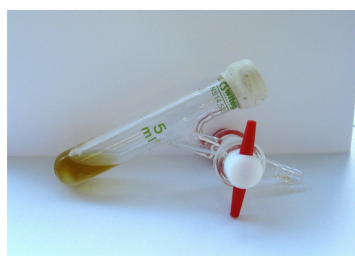
P((FGE 14 -co-GME 6 )C) and crosslinker in DMF before DA Reaction → Liquid solution
