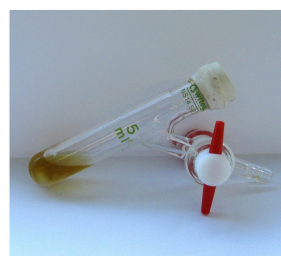
P((FGE 14 -co-GME 6 )C) and crosslinker in DMF after Retro DA Reaction → Liquid solution
