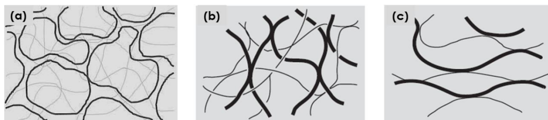
Fig. 3.5 Schematic models of the idealized structures in multicomponent gels. (a) Filled phase separated gel showing the example of a starch gel. (b) Mixed gel with two interpenetrating independent networks. (c) Complex gel with direct association between the polymer networks. Reprinted from [16].
