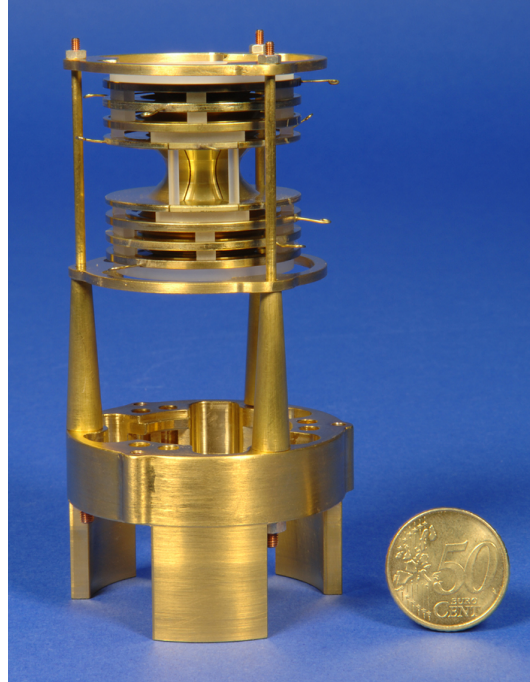
Figure 7.3: High-precision hyperbolic Penning trap for the cyclotron frequency determination. It is specially designed to improve the detection of the induced image currents (see text for more details).
