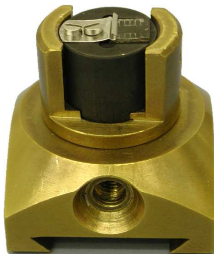
Figure B.2: Proper adjustment of the FIB sample in the SEM holder.
