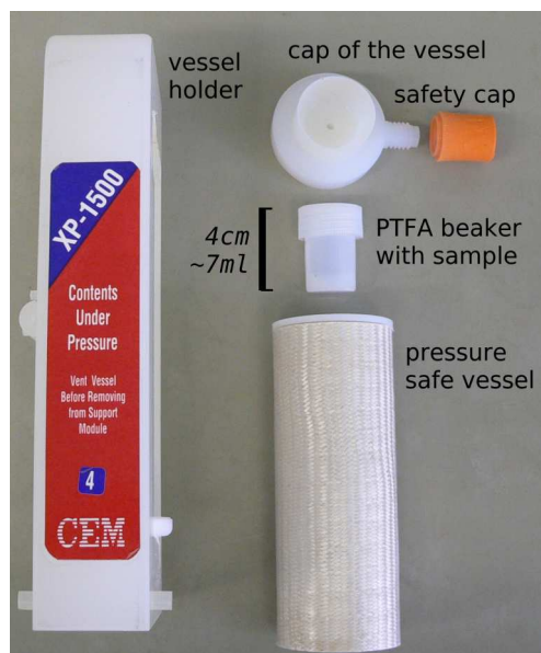
Figure 1: Detail for the assembly of the vessels for the microwave assisted digestion. PTFE beakers containing the sample and acid are introduced to the pressure safe microwave vessel. HCl is added outside the beaker to the vessel to ensure pressure equilibrium.
