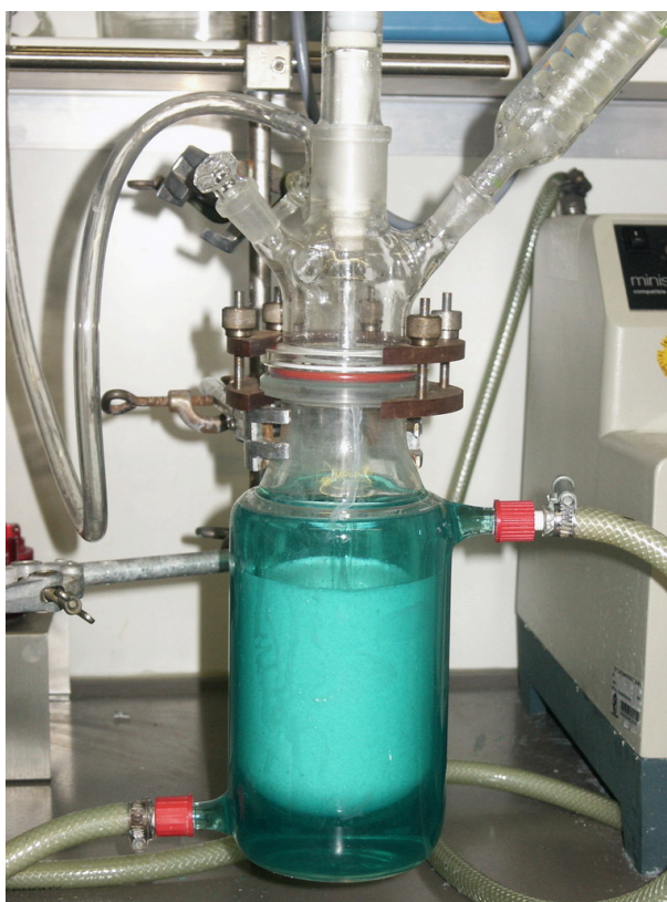
FIG. 4.1: Typical reactor used for synthesising a dispersion.
