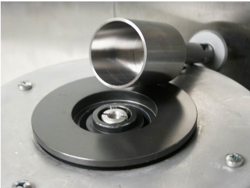
FIG. 3.4: This picture shows a double wall Couette.
