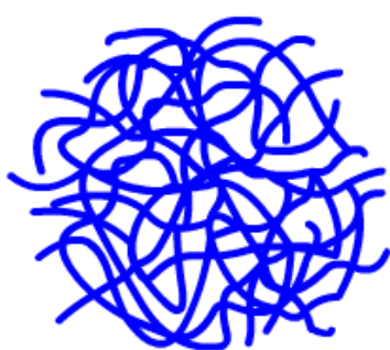
a) Polymer molecules in the solid state just after being added to a solvent
