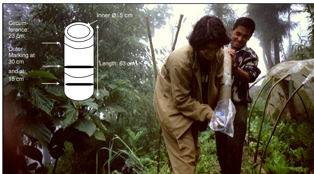
Fig. 4.18 & Photo 4.24: Soil sample equipment and taking of soil samples, Darjeeling District (Photo by SHILPI SAXENA, 2002)
