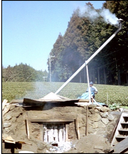
Photo 5.31: Kiln to make charcoal and wood vinegar, Shizuoka Prefecture (Photo by SHILPI SAXENA, 2003)
