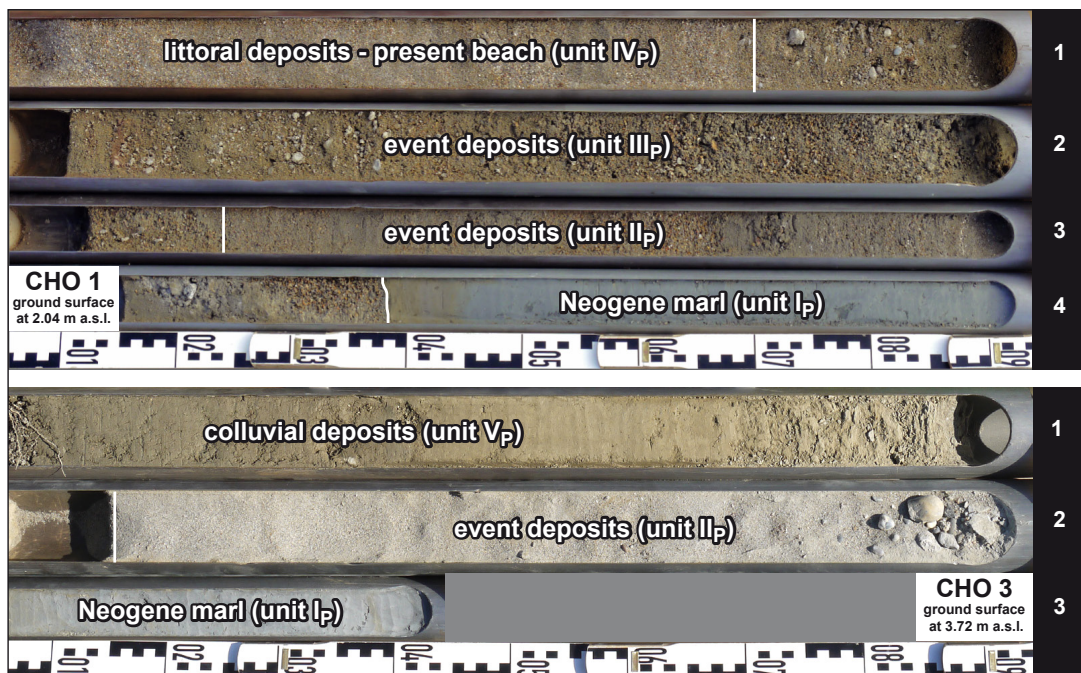
Fig. 2.9: Sediment cores CHO 1 and CHO 3 drilled at the present-day beach and in the middle of the Palaiochora promontory, respectively. For further information on sedimentary units see text.
