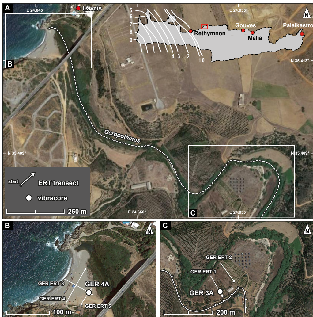
Fig. 4.1: Overview of the lower course of the Geropotamos River and the river mouth area into the Cretan Sea (A). Detail maps of the Geropotamos River mouth area (B) and the inactive external bank further inland (C) show locations of vibracoring sites and ERT transects. Isolines in inset map of Crete depict amount of coseismic uplift associated with AD 365 earthquake in meters (after KELLETAT 1991; SHAW et al. 2008). Maps based on Google Earth 2017.
