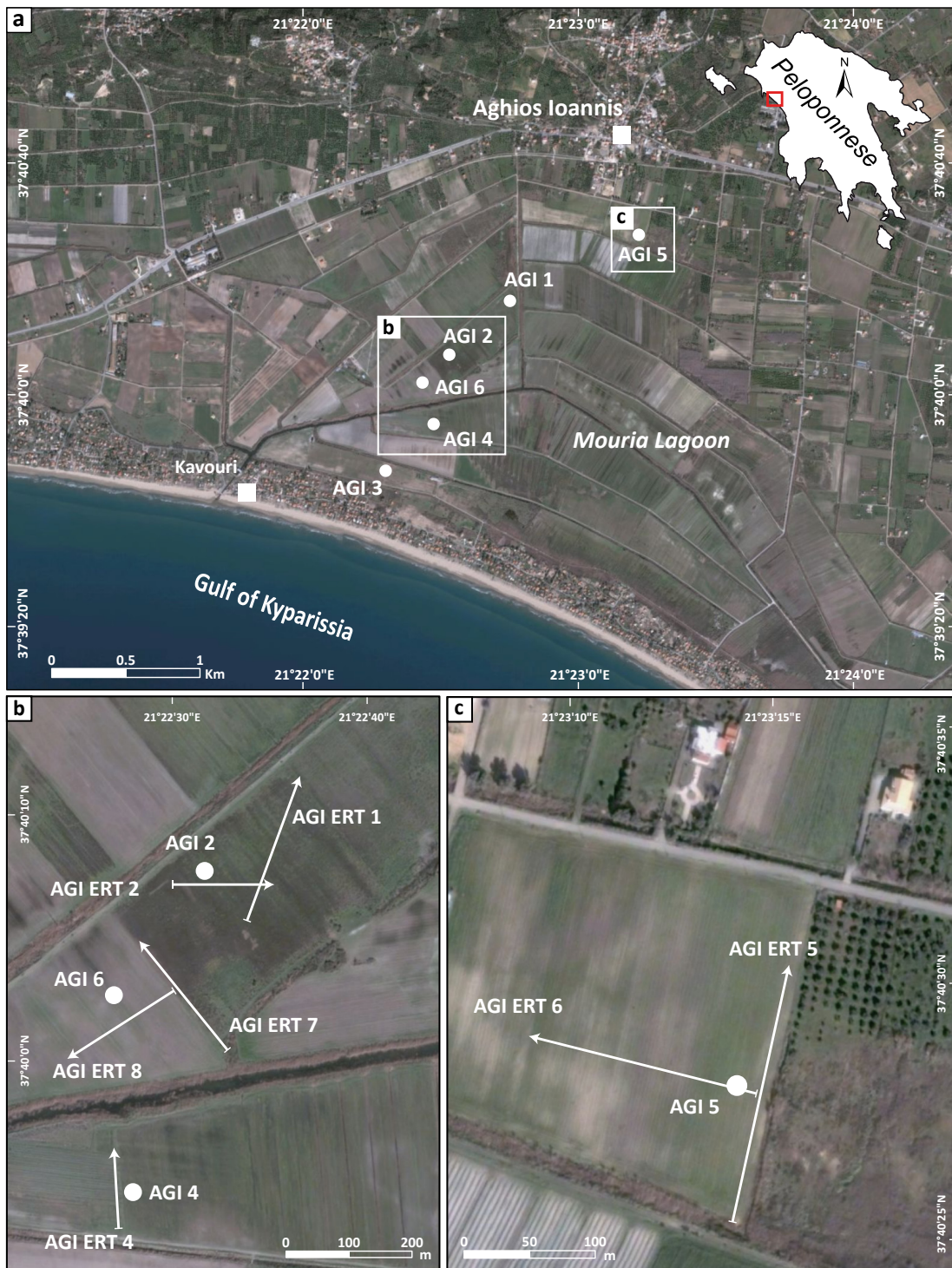
Fig. 3-2: Overview of the Mouria Lagoon (a), and detailed view study sites (b, c). Vibracore locations are marked by white dots and electrical resistivity transects are shown as white lines with measuring-direction (maps modified after Bing Aerial Maps, 2013).
