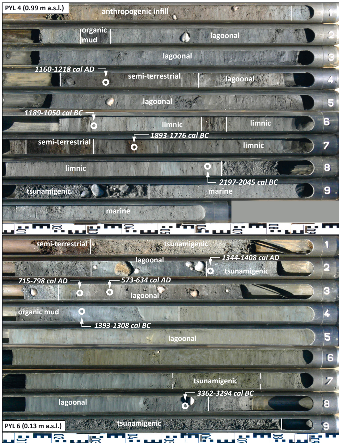
Fig. 4-4: Simplified facies profile and tagged radiocarbon datings of vibracores PYL 4 and PYL 6 drilled in central part and eastern end of the Voidokilia Dunes (for location see Fig. 4-2, details of radiocarbon datings are shown in table 4-1. At photo PYL 6, meter 9-10 is missing because of core loss.
