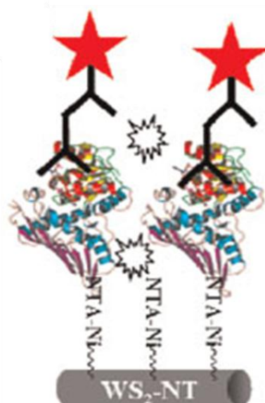
Figure 1.11. Schematic representation of the fabrication of biotitania/NT- \text{WS}_2 nanocomposite.
