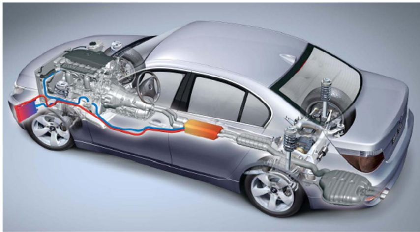
Figure 2 TE generator embedded into a BMW I
