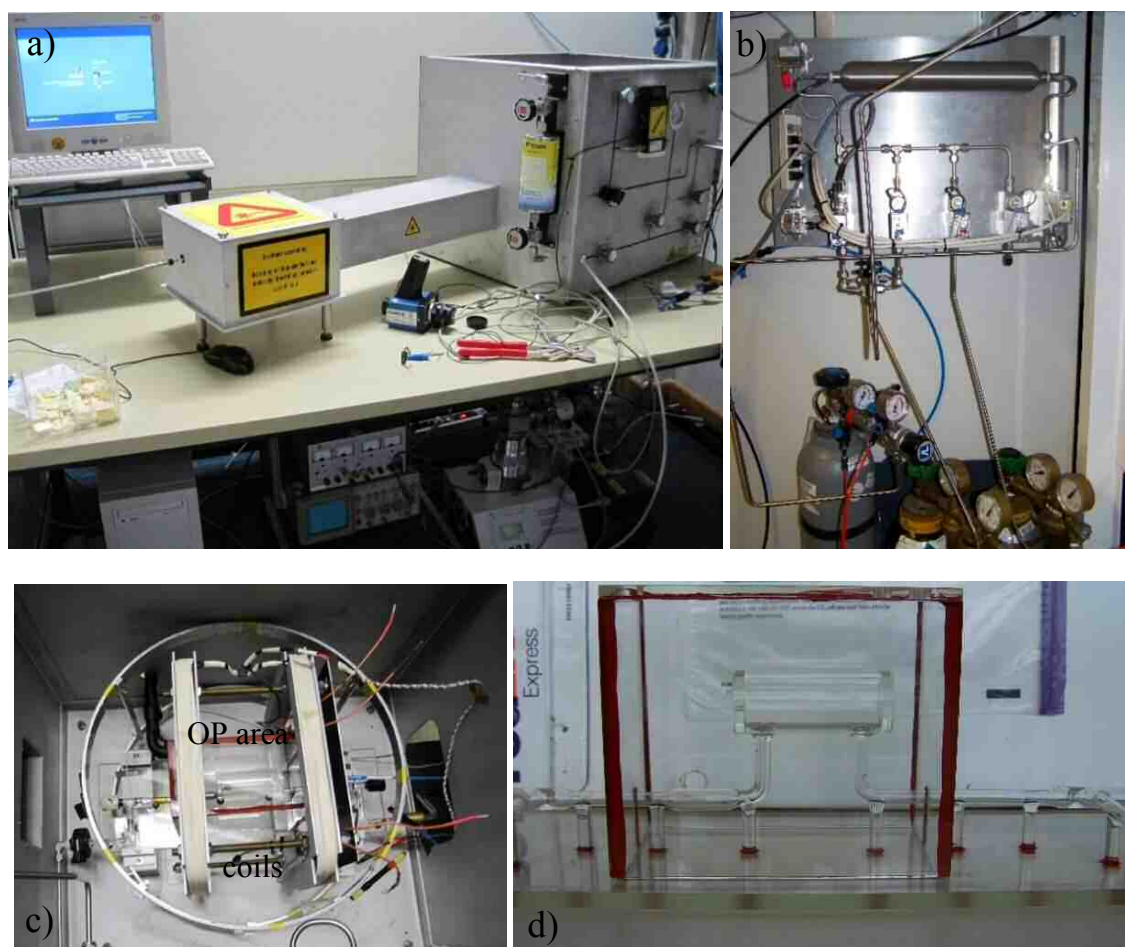
Fig A5.1: a) Photograph of the MPIP Xe-polarizer. b) Gas mixing panel and gas bottles fix to the wall of the lab. c) SEOP area. d) Optical pumping cell and oven.
