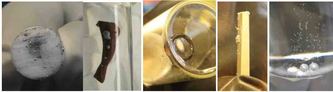
Fig. A4.2: Samples after the contact with Rb. From left to right: Teflon, silicon glue, FKM o-ring, piece of PEEK and silicon oil. The Teflon absorbed the Rb, in the grey regions, the material has a rubber consistency. In the silicon glue, the drops of Rb are printed on the surface when the Rb is removed. The o-ring did not show mayor changes after 6 months and PEEK as well. The reaction with silicon oil was really slow even at temperatures of about 80°C. The diameter of each Rb drop is about 5 mm and the bubbles are hydrogen gas.
