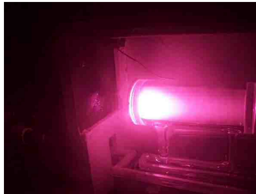
Fig 4.16: OP-cell filled only with Rb and illuminated with laser light at \lambda = 795 nm. The emitted light can be analyzed with an optical or digital spectrometer to verify the purity of Rb.
