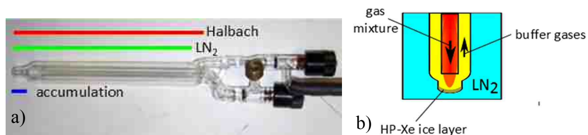
Fig. 4.30: Cylindrical accumulation cell. a) Picture of AC1. The red line indicates the part the cell inside the Halbach. The green line indicates the part of the cell submerged in LN 2 and the blue line indicates the part of the cell available for accumulation. b) Sketch of the accumulation area. The gas mixture flows through the inner tube and the HP-Xe freezes on the bottom part of the appendix. The buffer gases (He and N 2 ) flow to the outlet of the cell.
