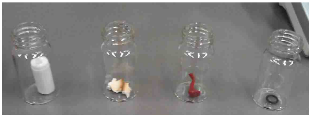
Fig. A4.1: Samples before the contact with Rb. From left to right: Teflon, epoxy glue, silicon glue and FKM.
