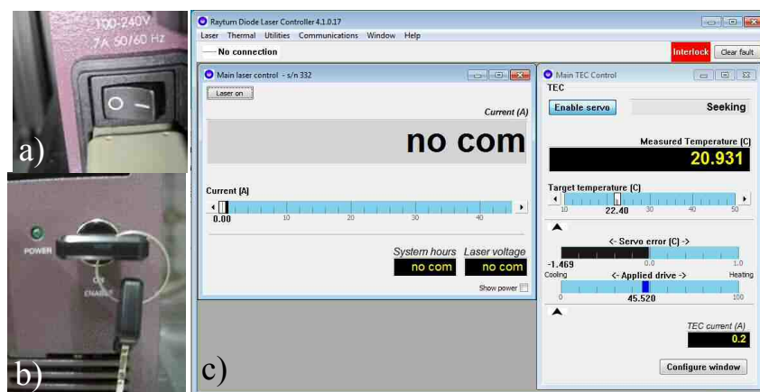
Fig. A3.3: Switching on the laser. a) Main switch. b) Safety key. c) Graphical interface of the laser.
