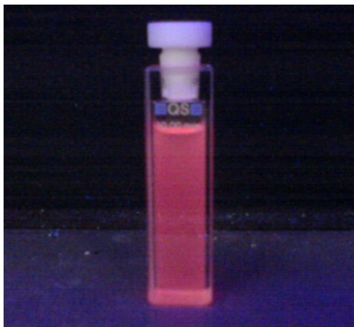
Figure 4-102: Picture taken from a sample of C_{72}-(C_{12})_4-(C_{14,10})_4-(t-Bu)_2 ( 4-119 ) dissolved in THF at room temperature and illuminated by an UV-lamp.
