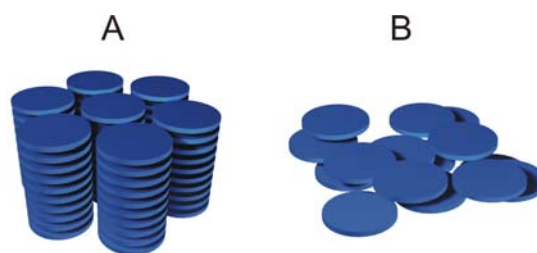
Figure 1-6: Illustration of the two different mesophases of discotic liquid crystals, (A) columnar, and (B) discotic-nematic.
