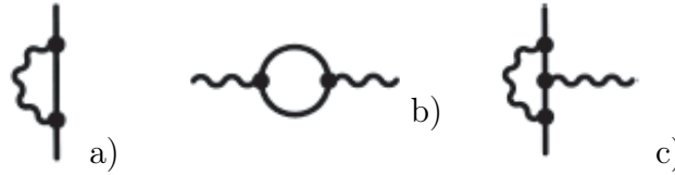
Figure 1.2: The basic quantum electrodynamical processes, represented as Feynman diagrams. The plain lines denote free electrons or positrons, the curly lines denote photons. (a) Emission and reabsorption of a virtual photon by an electron, the so-called self energy . (b) Creation and re-annihilation of a virtual electron-positron pair by a photon, the so-called vacuum polarization . (c) Modification of a basic electron-photon interaction by an additional virtual photon, the so-called vertex correction .
